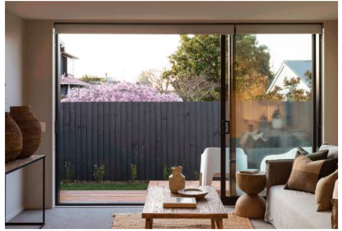
Double glazed windows with blinds for solar control and heat loss reduction, feltexgreen carpets for warmth and environmental sustainability.
